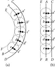
Huygens geometrical construction for the propagation of (a) spherical, (b) plane wavefront.
