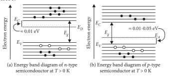
In *n*-type extrinsic semiconductors, the number of free electrons in conduction band is much more than
